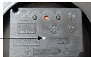
After receiving the time signal DCF and its internal processing (5 to 10 minutes), the clock is automatically set to the time
